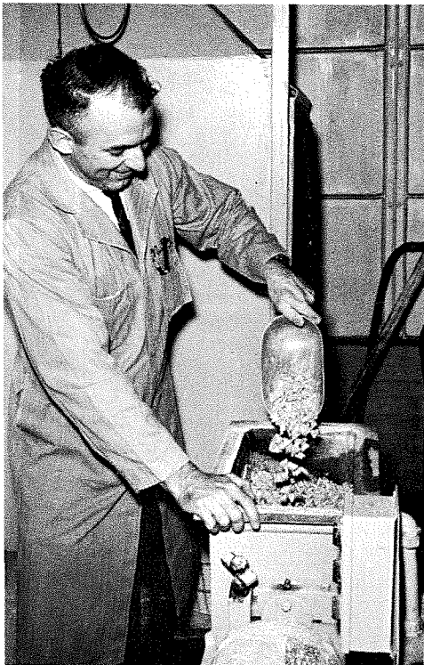
Performing a media test is chief chemist Norm Roy. Tests are made to compare competitive media with ours. Media is used in Lorco vibrators for a number of precision finishing jobs.
