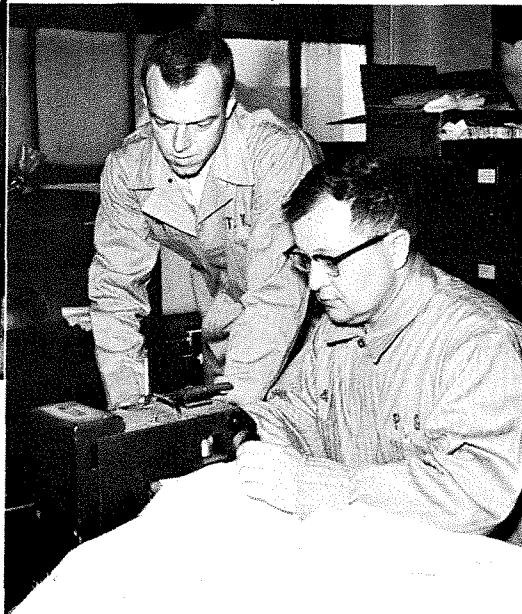
Tom Bodle and Paul Kohler test cloth as part of their duties as Dust & Fume technicians. Cloth is integral part of the collecting system as it must restrict the passage of contaminants while filtering air.
